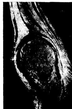
Figure 5. Petroleum pyrolytic electrode coke; magnification \times 49 .
