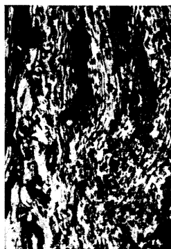
Figure 7. Pitch electrode coke; magnification \times 350 .
