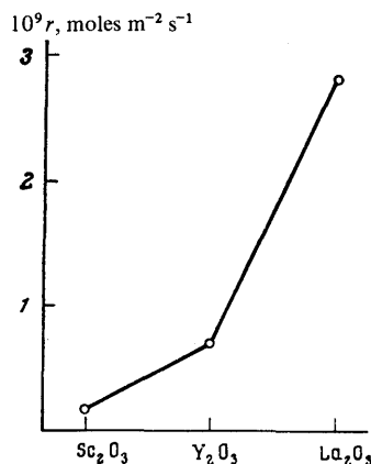
Figure 4. Activity of oxides of the scandium subgroup in the hydrogenation of ethylene at -78^\circ\text{C} .
